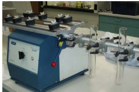
Figure 1. Laboratory wrist-type shaker used to test egg and larval quality relative to physical stress.
